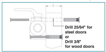
Note 1: For Through Bolts, specify door thickness if other than 1 3/4" (44 mm).
